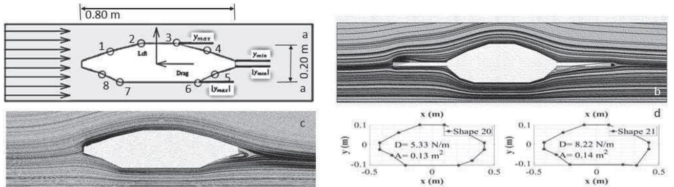
Fig. 5 2D hybrid optimization and CFD simulation; a) general dimension and selected points for the optimization; b and c) fluid flow around the generated shapes from the optimization; d) Exemplary calculated drag forces for generated shapes
