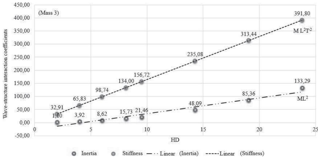
Fig. 7 Inertia and hydrostatic coefficients
