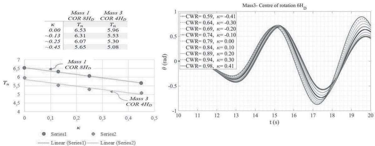
Fig. 9 Parametric study of PTO stiffness, mass, and center of rotation.
