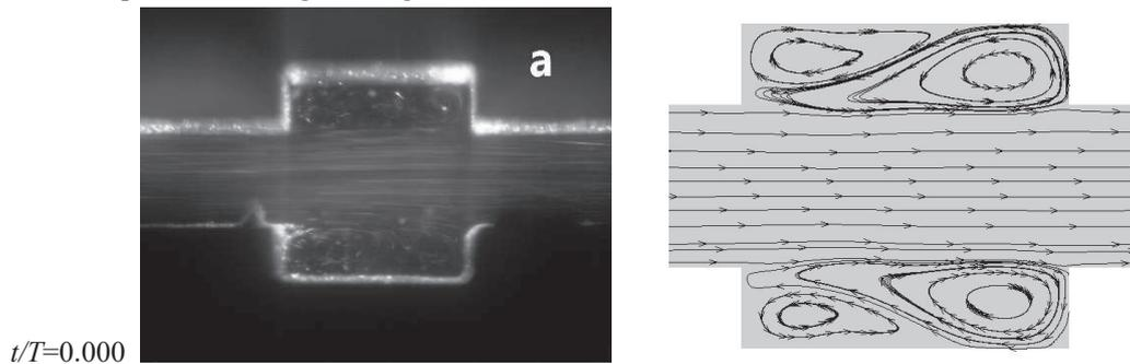
Fig.3.1 Comparison of fluid morphology and numerical simulation results
