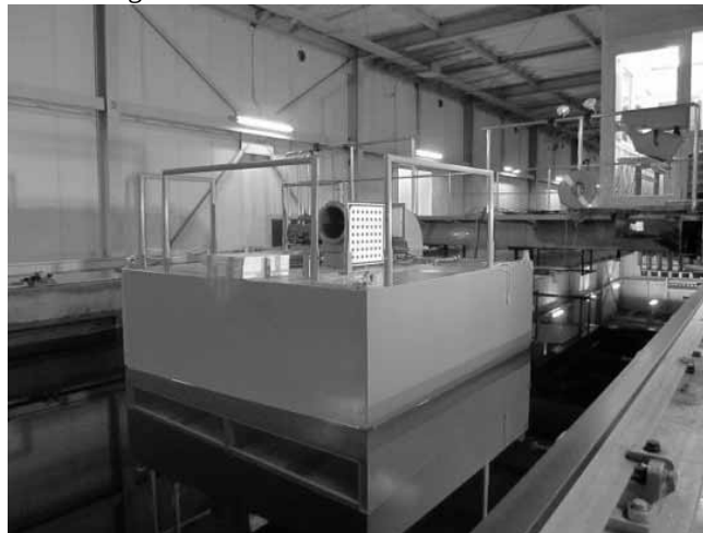
Fig.4 BBDB model installed in a tank
