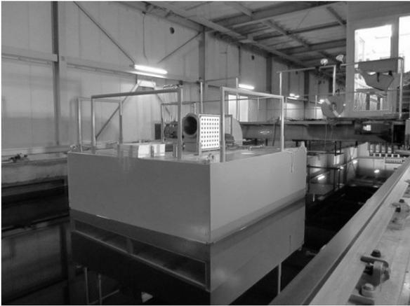
Fig.19 Turbine attached BBDB
