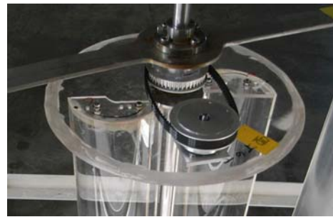
Fig. 16 Ratchet mechanism attached on the Savonius rotor
